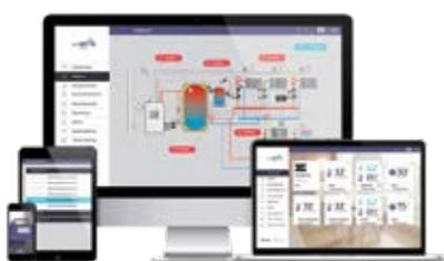
The ecoNET internet module ensures remote access to the controller by such devices as PC, tablet or smartphone. The user has the ability to adjust basic controller parameters influencing operation of the whole
